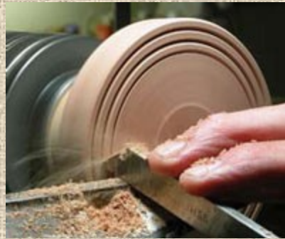
Photo 1: Use a beading tool to cut three beads into the rim of the medallion.
