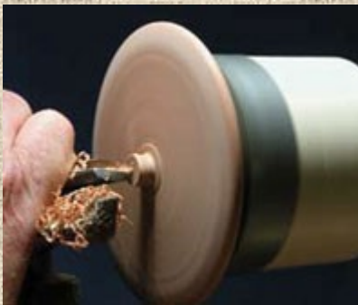
Photo 4: Back off the tailstock and carefully turn away the remaining small tenon.
